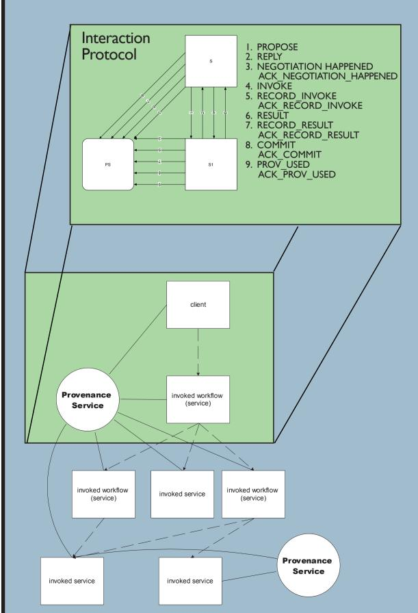
The PASOA architecture is an asynchronous mechanism for recording provenance. The architecture is designed to work with multiple provenance services, as well as multiple workflow enactment engines, i.e. a client calls a workflow enactment engine which then calls a variety of services some of these services (workflow enactment engines) may in turn call other services until a result is returned up the hierarchy.
