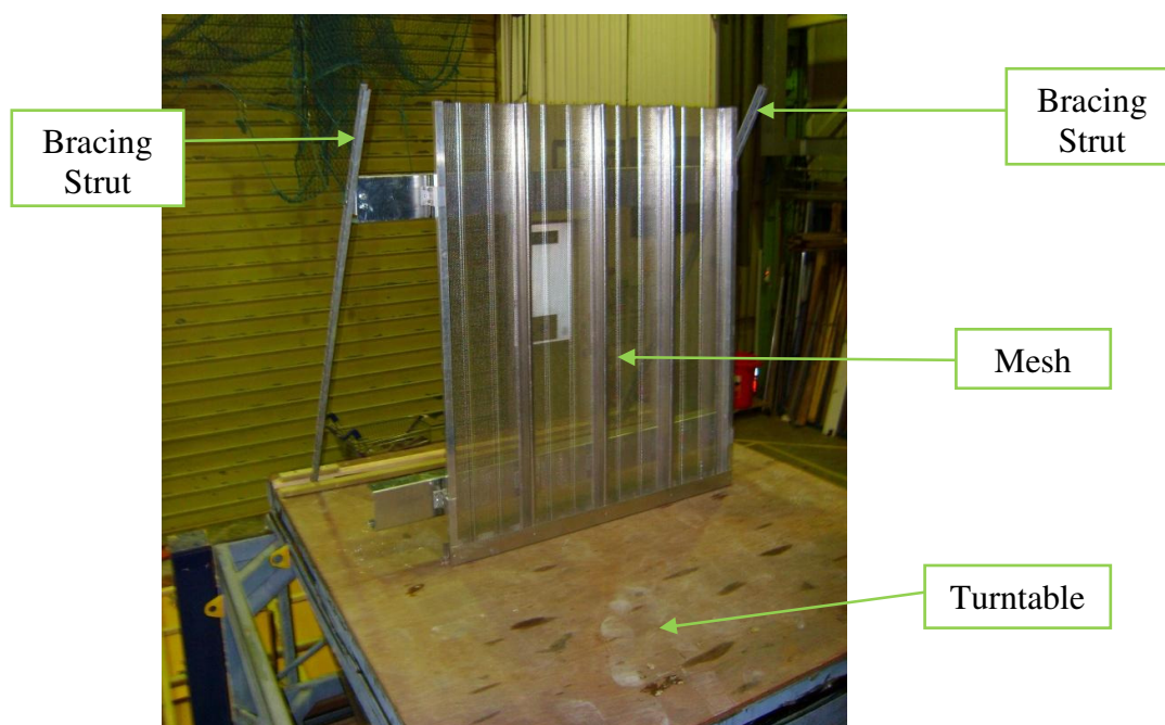
Figure 1. View Looking From Wind Tunnel Outlet Towards Mesh
