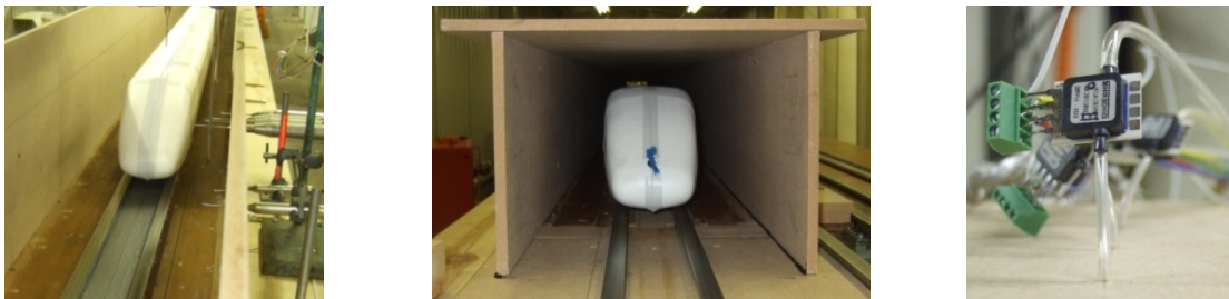
Fig 1: Left: Walls (Cobra probes visible). Centre: Walls & Ceiling. Right: Pressure tappings.
