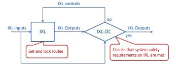
top of existing interlocking systems while still providing a provably safe interlocking system.
