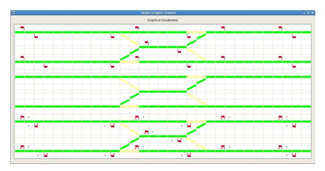
The figure below shows that two routes with their overlaps have been booked (red line sections), that their entry signals are open (green boxes) and that two trains has entered these routes (black line sections). It shows also that the dynamic controller is not aware yet that the trains passed the entry signals of the routes.
