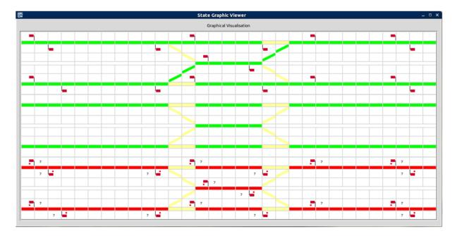
The figure below shows the state of the dynamic controller after the point sensors have being fixed and the dynamic controller has got the state of the sensors. So the dynamic controller considers all track sections free and all points controlled in left position.
