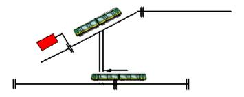
These two properties have been merged into a single property that corresponds to the incompatibility between the blocks, as defined by the property below. We check that two different trains do not intersect in an incompatible area. This area includes the fooling area and the face to face area.
