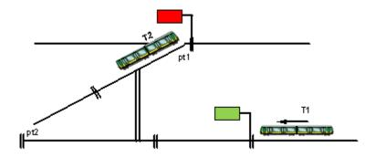
Furthermore, consideration of trailable points has not been retained. Indeed, these points can change position during the passage of a train, as illustrated in the figure below. In this example, the point is right before train passage, and then train changes the position of the point to the left.
