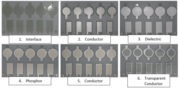
Figure 3: 6 individually printed layers built up to produce EL display.
