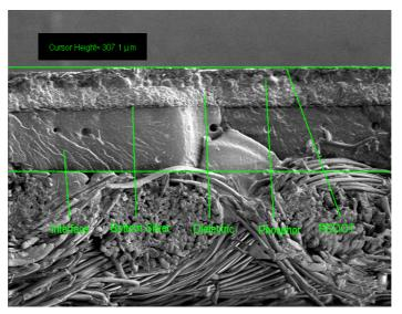
Figure 4: SEM micrograph showing EL lamp cross-section.
