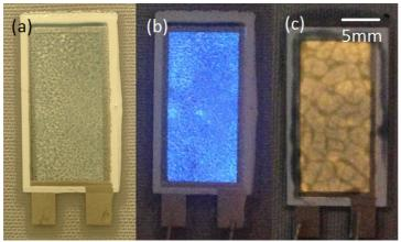
Figure 1: Screen-printed EL samples on fabric (a) Unpowered, (b) Dark blue powered, (c) Orange powered.
