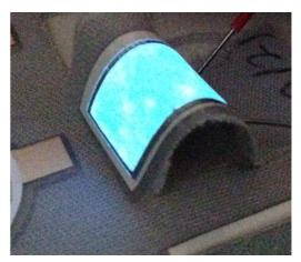
Figure 2: Screen-printed light blue EL lamp on fabric showing maintained fabric flexibility.
