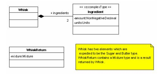
Figure 8 The UML model of the Whisk messages
