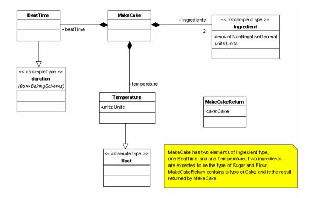
Figure 7 The UML model of the MakeCake messages
