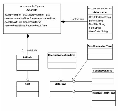
Figure 12 The UML model of actor provenance data
