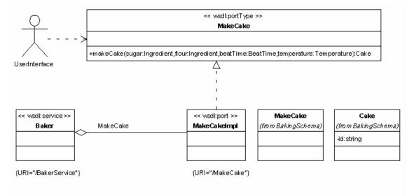
The UML model of the Baker service is shown in Figure 13.
