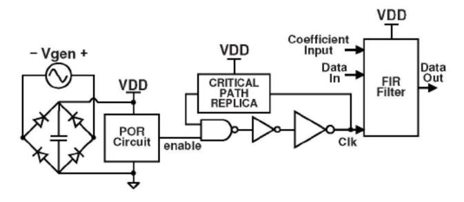
Fast Power-on Reset (4.1nW), 3T DRAM to keep state across supply cycles, 135K transistors in 180nm CMOS Can supply 250KHz on all process corners for <=50C
