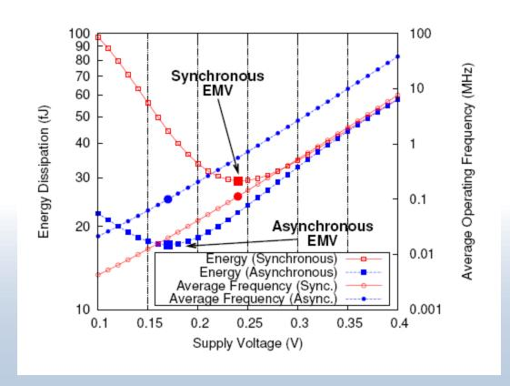
Asynchronous (self-timed) logic can provide completion detection and thus reduce the interval of leakage to minimum, thereby doing nothing well!
