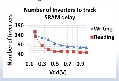
For example, under 1V Vdd, the delay of SRAM reading is equal to 50 inverters and under 190mV, the delay is equal to 158 inverters
