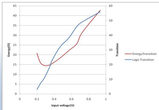
Energy and transition count vs different Vdd samples into the Capacitor
