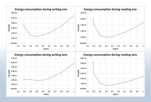
The curves show that the minimum energy point of the chip is at 400mV-500mV.
