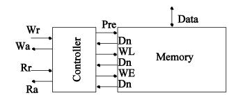
The SI controller uses completion detection in SRAM and handshake protocols to manage pre-charge, WL and WE in the SRAM banks
